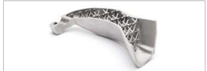
Fig. 2: Part structure with load-adapted supports
