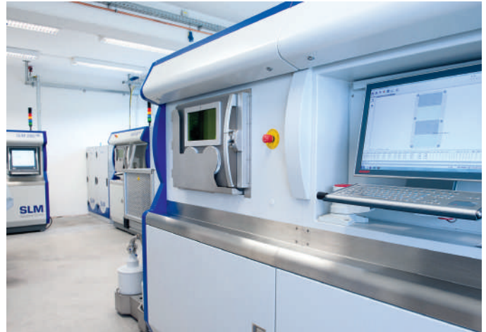
Fig. 1 Additive Manufacturing using SLM®280 and SLM®500 machines at Rolf Lenk
