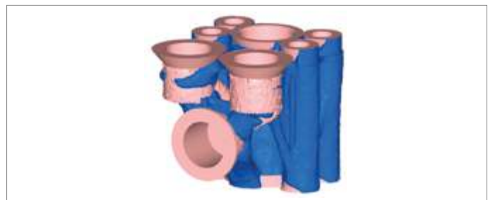
Fig. 2: Interpretation and remesh of topology optimization result
